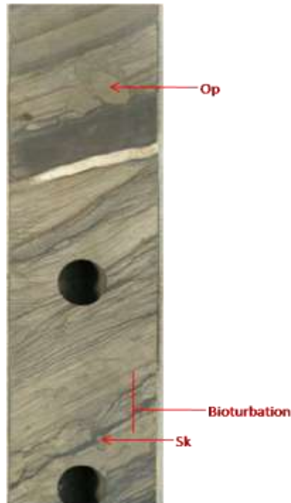
Figure 9: Boga Well-5 (Depth 3698.3—3698.8) Reservoir “A1”: Op: Ophiomorpha ; Sk: Skolithos
